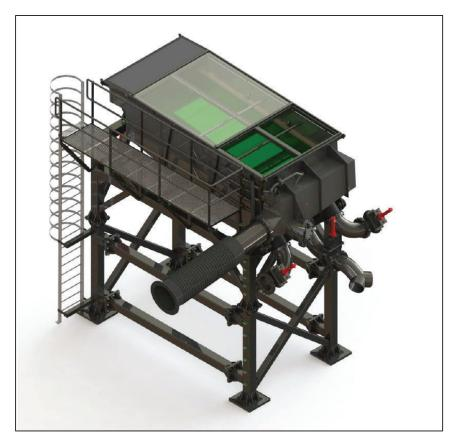
Figure 2-3: Diagram of sand "Screening Deck" on the 'William Fraser'
